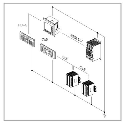
Remember that the ground terminals of all the elements making up the system must be connected to a single ground point.
