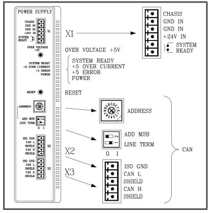
X1 Chassis For system ground connection. X1 +24V / GND For the 24 Vdc power supply. For the emergency chain from the electrical cabinet. X1 System Ready It is an internal contact that closes when the group is
