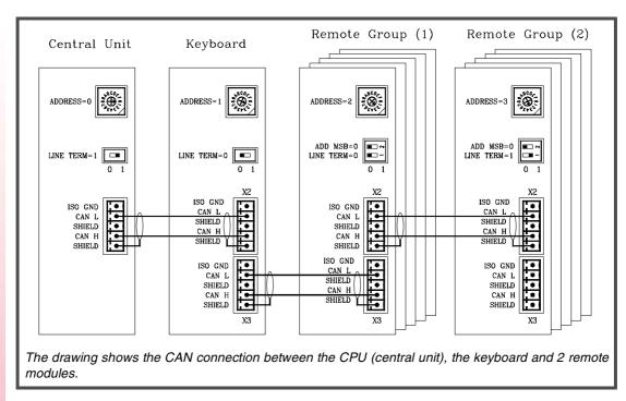
Respect the cable's minimum bending radius when connecting it. See "CAN cable characteristics."
