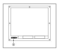
**A.** Connector for the CPU keys with the CNC keyboard. Maximum cable length is 1 meter.
