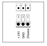
3-pin male Phoenix minicombicon connector (3.5 mm pitch).
