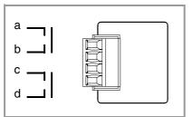
They are two normally open contacts that close when the CNC is turned on and it is running properly. They open again when turning the CNC off or due to an internal failure
