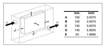
To ensure the required ambient conditions, the enclosure must have an air input next to the cables and an air output next to the fan. In this case, install fans to ventilate the enclosure and keep the temperature within the allowed limits.
