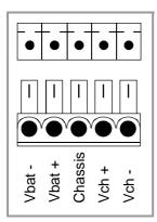
5-pin male Phoenix minicombicon connector (3.5 mm pitch).
