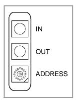
It is used to communicate with Fagor digital drives.
