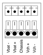
5-pin male Phoenix minicombicon connector (3.5 mm pitch).
