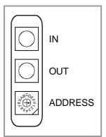
It is used to communicate with Fagor digital drives.
