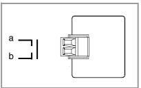
It is a normally open contact that closes when the CNC is turned on and it is running properly. It opens when turning the CNC off or due to an internal failure
