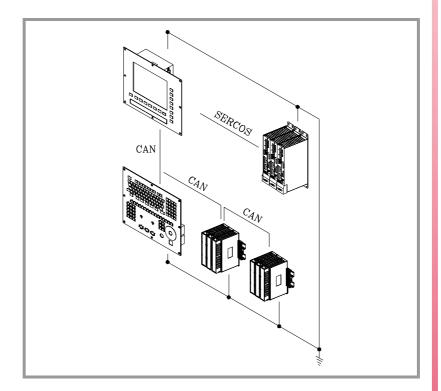
Remember that the ground terminals of all the elements making up the system must be connected to a single ground point.
