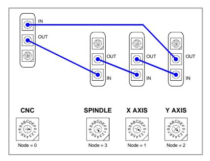
The drawing shows the SERCOS® connection of the CNC with Fagor spindle drives and the X, Y axes.
