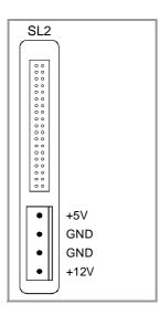
For connecting a CD-ROM drive or another device that uses an IDE interface to the central unit.
