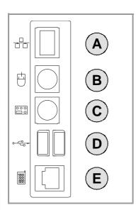
With the CPU board, it is possible to connect the most common PC peripherals, even a modem, to the CNC. It also has an Ethernet connector to integrate the CNC into a network.
