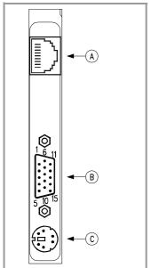
The CPU board allows connecting the unit to an Ethernet network. It also allows connecting the following peripherals to the unit.
