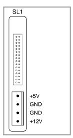
For connecting a floppy disk drive to the central unit using the floppy disk interface. See "13 Floppy disk drive.".
