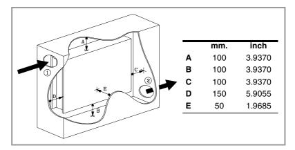
To ensure the required ambient conditions, the enclosure must have an air input next to the cables and an air output next to the fan. In this case, install fans to ventilate the enclosure and keep the temperature within the allowed limits.
