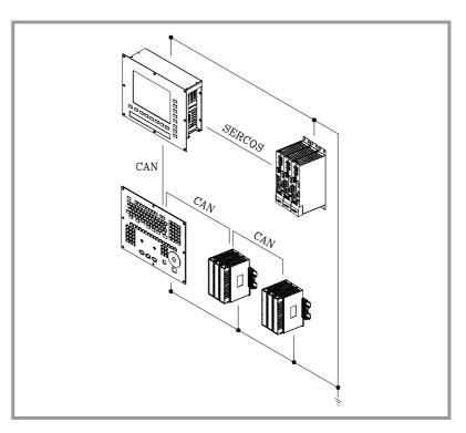
Remember that the ground terminals of all the elements making up the system must be connected to a single ground point.
